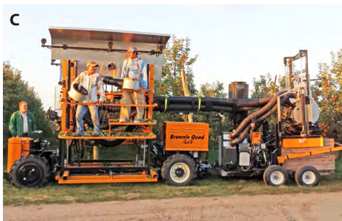
Figure 1. Commercial self-propelled apple harvest assist platforms: A. Flow Thru Harvester, Precise Manufacturing, Inc. (Photo courtesy Precise Manufacturing, Casnovia, MI); B. Huron Fruit Systems, Wafler Farms (Wolcott, NY). C. DBR Vacuum Harvester, Phil Brown Welding Corp. (Conklin, MI); D. Pluk-O-Trak Apple Harvester, Munckhof (The Netherlands). (Disclaimer: Mention of commercial products is only for providing factual information for the reader, and does not imply endorsement of the products by USDA over those not mentioned.)
