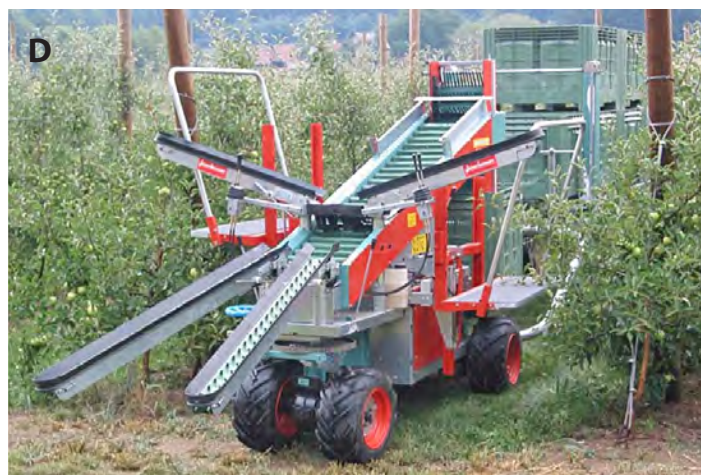
Figure 1. Commercial self-propelled apple harvest assist platforms: A. Flow Thru Harvester, Precise Manufacturing, Inc. (Photo courtesy Precise Manufacturing, Casnovia, MI); B. Huron Fruit Systems, Wafler Farms (Wolcott, NY). C. DBR Vacuum Harvester, Phil Brown Welding Corp. (Conklin, MI); D. Pluk-O-Trak Apple Harvester, Munckhof (The Netherlands). (Disclaimer: Mention of commercial products is only for providing factual information for the reader, and does not imply endorsement of the products by USDA over those not mentioned.)
