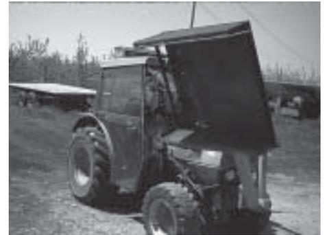
Figure 6. Flamer raised for easy transport and repairs or adjustments.
