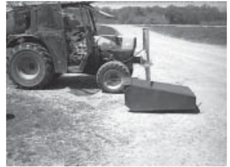
Figure 3. Flamer mounted on front of tractor.
