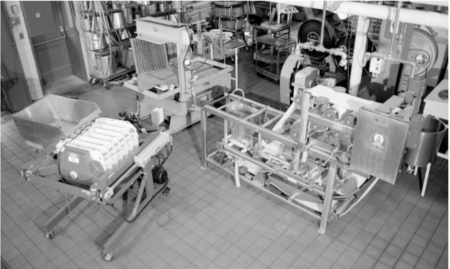
These fruit and vegetable presses are located on the floor of the Fruit & Vegetable Processing Pilot Plant at NYSAES, and available for use by FVC clients. From left to right: Good Nature Accordian, Orchard Equipment Rack & Frame, and Frontier Continuous Belt.
